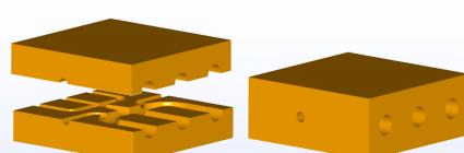
Macro-heat exchanger, z.B. ITER, t~14mm
