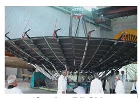
"Spektr-R" SV: dimensionally stable antenna structures for the radio telescope
